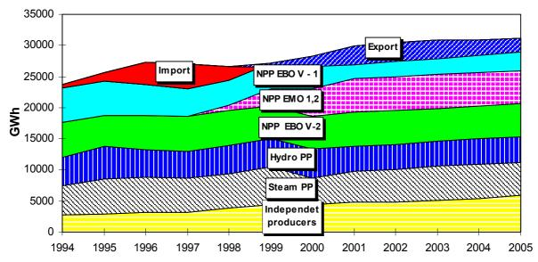
Fig. 5. Development of Electricity Generation
